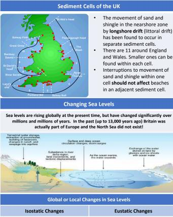
The movement of sand and shingle in the nearshore zone by longshore drift (littoral drift) has been found to occur in separate sediment cells. There are 11 around England and Wales. Smaller ones can be found within each cell. Interruptions to movement of
