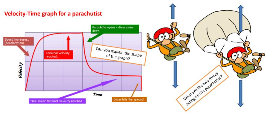
When an object starts to fall, the resultant force is in the downwards direction due to the weight causing the object to accelerate. As the object accelerates the resistive force increases. Eventually the two become equal but opposite (there is no resultant force) so the object starts to travel at a constant velocity, this is known as the objects terminal velocity.
