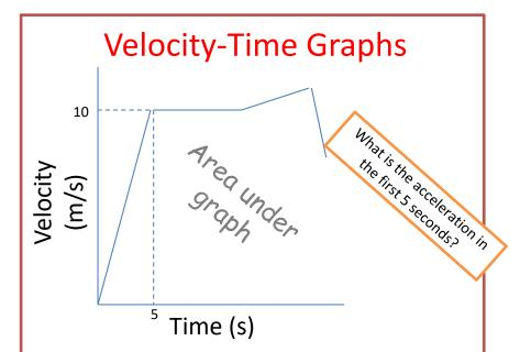
The gradient gives you the acceleration of the object. The steeper the line the greater the acceleration.
