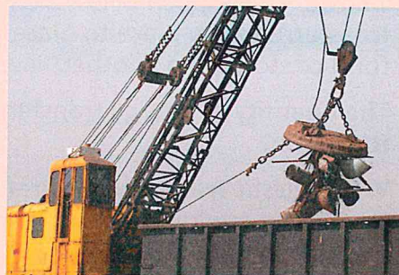
FIGURE 2.2.7a: Using an electromagnet in a scrapyard.
