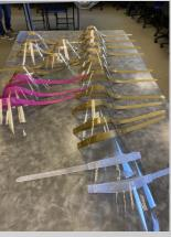
The original 2D design, shared by Sandbach School, was tweaked to maximise production on CHS machines, enabling 60 full headsets to be produced per hour. Two laser cutters created each of the three sections of the headband, then the clear screen was guillotine cut and shaped with scissors. Before constructing the visor by hand, each component was sanitised. The completed visors were then
