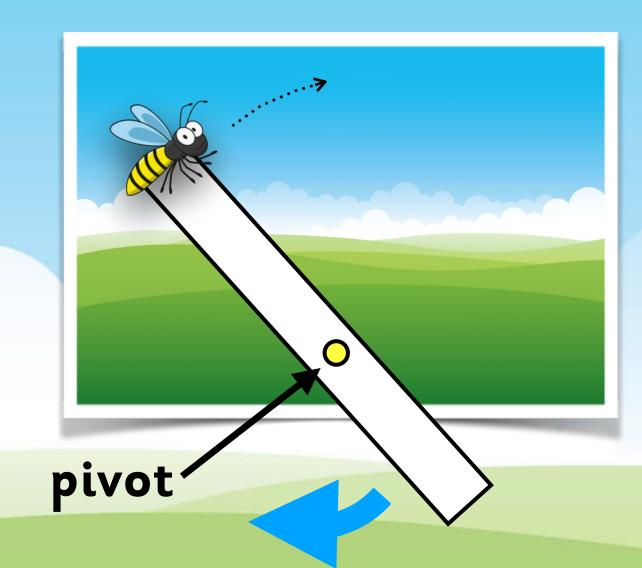
The **pivot** is made by making a hole in the lever and the background scene, and inserting a paper fastener to join them together.
