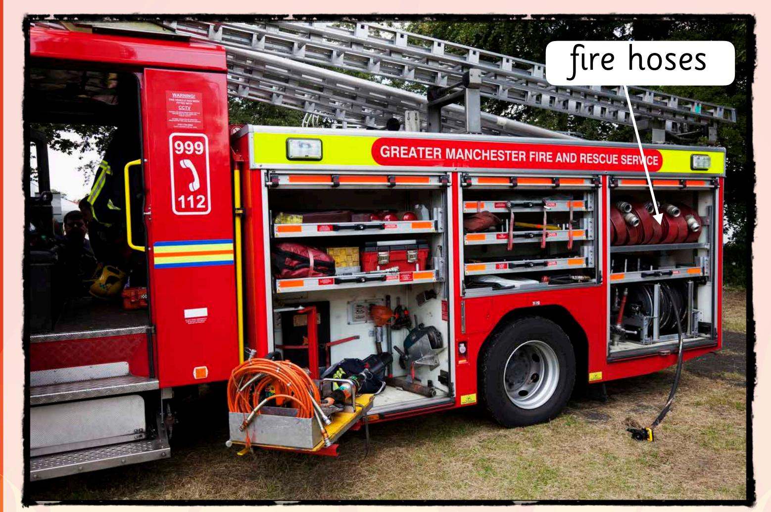
Fire engines need lots of special equipment to help them fight fires and carry out other rescues. Fire hoses attach to the water tank in the fire engine so that the firefighters can spray a fire with water to put it out.
