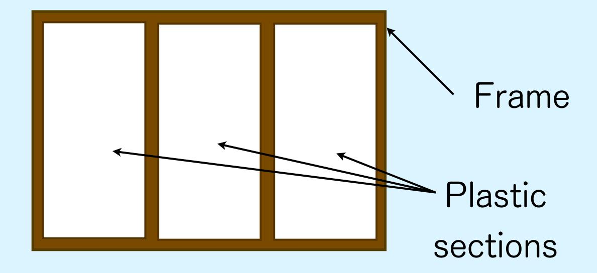
This structure has a **thick** frame. The sections of plastic are **small** so the stability of the frame is **stronger**. However, **less** sunlight can enter the greenhouse.
