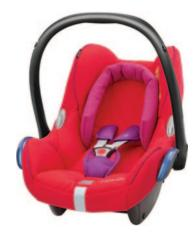
\*IsoFix - A child car seat attachment system which uses compatible metal connection points on the car and the seat. It is designed to make installing a car seat quick and easy. It removes the risk of incorrect fitting when using the car's seatbelt to secure the seat.
