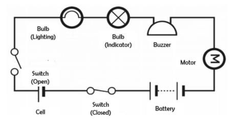
When drawing electrical circuits, you should use the standard symbols to show the different components.
