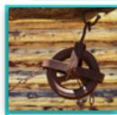
Pulleys A pulley is a wheel over which a belt, rope, or chain is pulled to lift or lower a heavy object.
