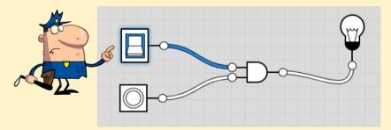
If the ON/Off Motion Switch detects movement it will switch to on (Input = 1) and the security light will turn on. This is shown below:
