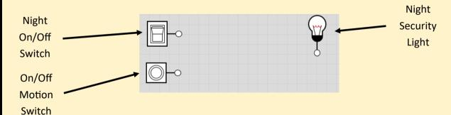
To get this to work we need to us and **AND** gate so the light only come on (Output = 1) when the Night ON/Off Swith is on (Input = 1) **and** the On/Off Motion switch is on (Input = 1).
