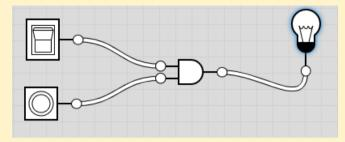
If the On/Off Motion Switch detects movement then it would switch to on (Input = 1). This is shown below:
