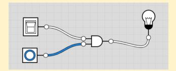
At night the Night ON/Off switch will be on (Input = 1). While there is no motion in the room the security light will not come on. This is shown below:
