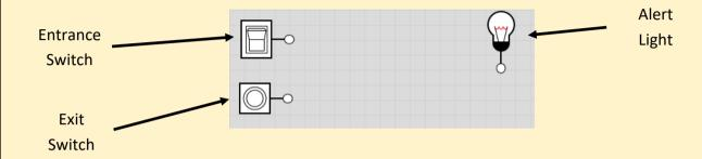
Now you want the light to come on when people are going in or out. This means that the light only comes on when the entrance switch is on **or** the exit switch is on.
