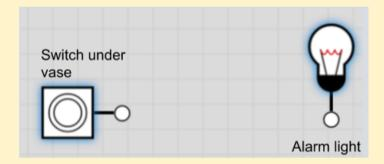
For this to work we need to use a **NOT** gate. A NOT gate changes its input. If the switch is on (input = 1) then the output will be off (output = 0) and vice versa.
