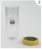
Turn the top part of the bottle upside down and place it inside the bottom part - fix it in place using the tape.
