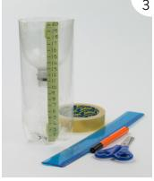
Make a scale in centimetres on a piece of tape, using a ruler, and fix it to the side of your bottle. You could sellotape a spare ruler on the side if you have one.
