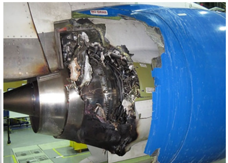
(The uncontained engine failure on the CS100(now the A220-100))
