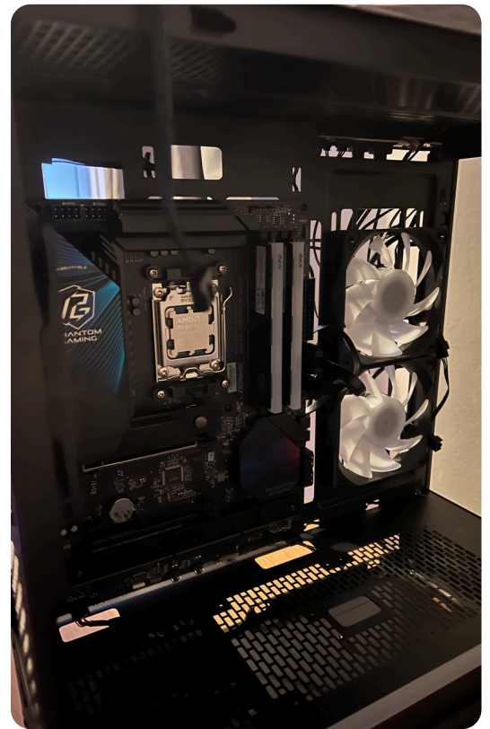
The motherboard after being installed into the case.
