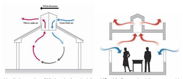
Passive Ventilation, such as "Windcatcher" on the left and "Stack" effect on the right, use a combination of natural convection and wind speed to draw fresh air in. They can also incorporate supply fans, to supplement supply air when wind direction or strength fluctuates and typically include external weather sensing, and automated controls. "As Installed Records" and Service Records should be reviewed to identify the type of system in use
