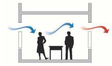
Cross Ventilation, could also draw fresh air from a central corridor or atrium. See Mechanical Supply Only below.
