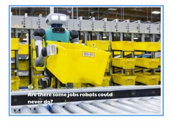
A new robot called Digit, designed to be humanlike and capable of lifting and moving items, is being tested in warehouses of the online retailer, Amazon. The robot is in its first few weeks of trials at Amazon's facility in Seattle, USA, as the company tries to improve automation in its processes. To begin with, the robot is being taught to pick up and move empty boxes to ensure that they are ready for reuse. The yellow boxes, or totes, are used throughout the company's fulfilment process.
