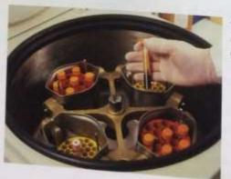
Figure 4 An ultracentrifuge used to separate the various components of cell homogenate
