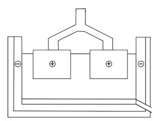
The positive ions are attracted to the negative electrode where they form aluminium atoms. Negative oxygen ions are attracted to the positive electrode where they react to form O2 molecules.
