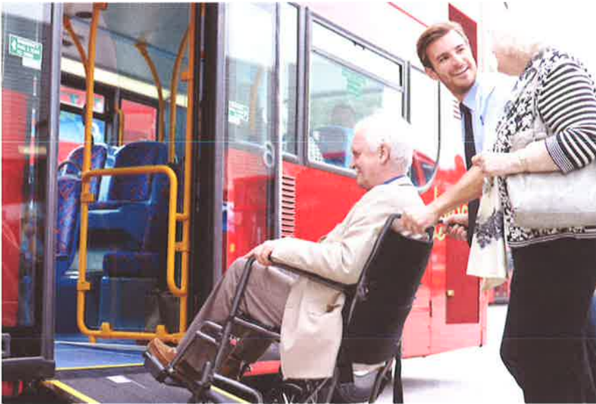
Figure 1.6 Providing a wheelchair ramp enables access
