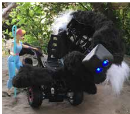
Bo Peep Figurine, standing proudly beside a real-life remote-control skunk mobile, made from 3D printed chassis and a plushy covering made from a textile template.
