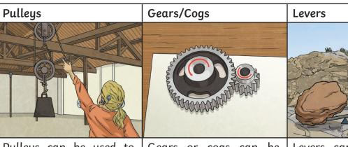
Pulleys can be used to make a small force lift a heavier load. The more wheels in a pulley, the less force is needed to lift a weight.
