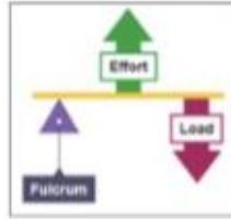
3 rd Class Lever: Force in the centre E.g. Lifting a dumbbell
