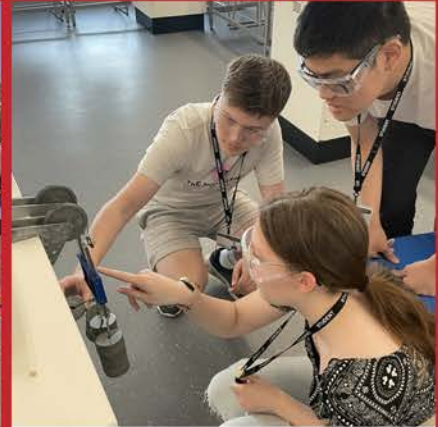
Our Year 12 Physicists have been practising using Vernier callipers to measure small stretches in wires in order to determine the Young's modulus of the wire. Great work all.
