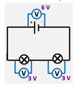
24. The voltage across the cell is equal to the voltage on each pathway of a parallel circuit.
