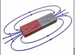
Magnets can be broadly categorised into two types, permanent and temporary. Permanent magnets can keep their magnetism for a long period of time, potentially for thousands of years. They have their own magnetic field due to the materials they are made from. Iron, cobalt and cobalt are the only elements that can show permanent magnetism. Man-made alloys such as steel can produce a stronger permanent magnetic field.
