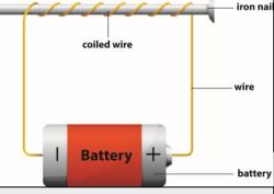
**Temporary magnets** are **only magnetic** when in the **presence** of another **magnetic field** and no longer show magnetic properties when away from that source. As an example, if you were to attach a paper clip or an iron nail to a bar magnet, then that nail or clip would be able to pick up another nail etc. **Electromagnets** are special cases where they are only **magnetic** when an **electric current** passes through the object.
