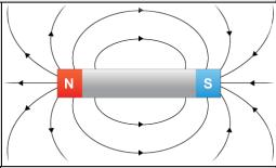
On an **electromagnet** at one end of the coil there will be a **north pole** and vice versa. If you **reverse** the flow of the **current**, the poles will **switch**.
