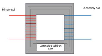
**change** the **potential difference** of an alternating current power supply.
