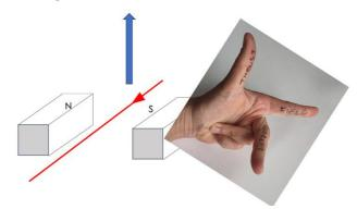
42. For a conductor at right angles to a magnetic field and carrying a current:
