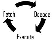
Once a cycle is complete, the CPU is ready to carry out the next cycle
