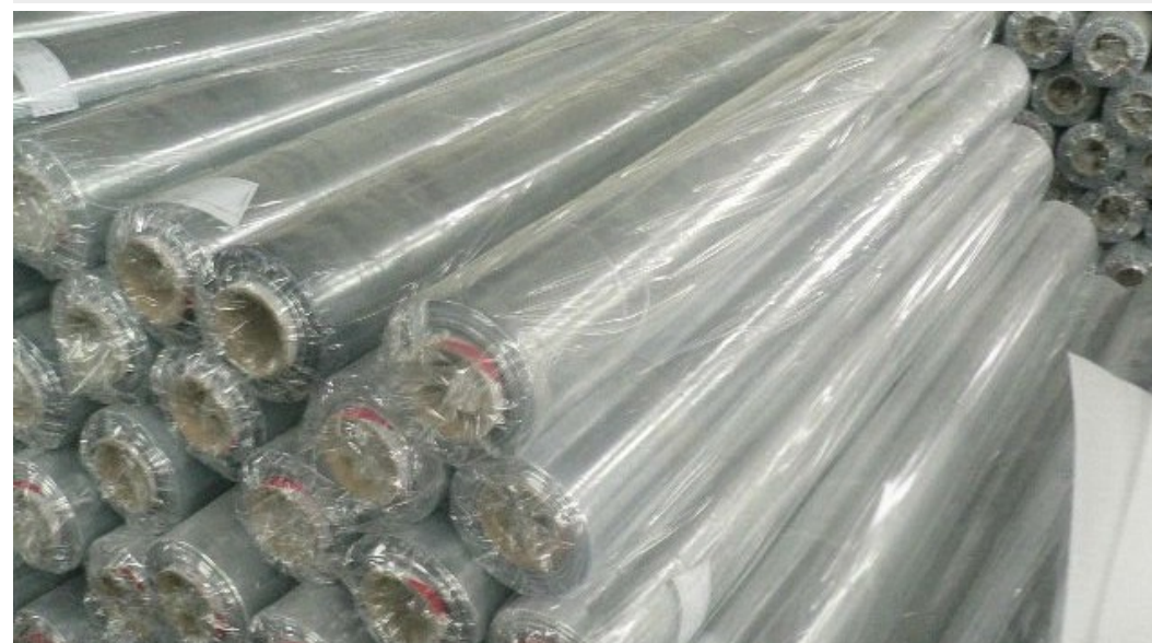
(above) PVC rolls produced by calendaring.
