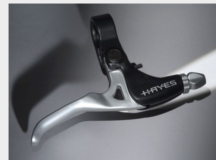
(above) A die-cast one-piece calliper brake lever for a bicycle.
