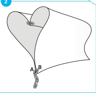
Curl the halves of the paper outwards and downwards and clip together the corners (A and B), which will be the front of the hang-glider. Attach a short chain of paperclips to the clip at the front (try varying the number).
