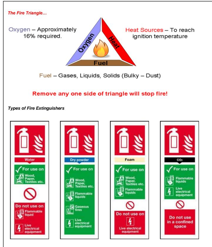
Please note that although  $CO_2$  is nonconductive, electrical equipment involved in a fire should always be isolated whenever possible before the extinguisher is used. Because of extreme cold (especially the discharge horn), only the squeeze grip control and carrying handle should be held during use.
