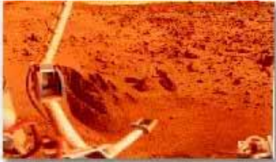
Viking 1 Lander sampling arm scooped up samples of Martian soil and put them into an instrument that studied them for signs of life. None were found.
